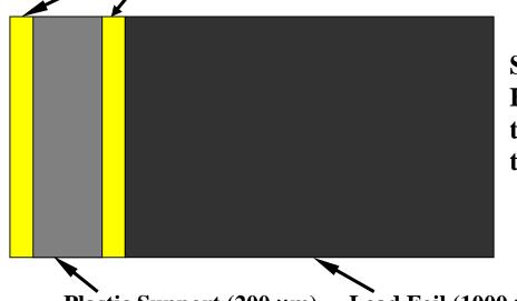
Set-up of a cell in the OPERA Experiment. 56 cells compose a brick, the fundamental unit of the OPERA target.
