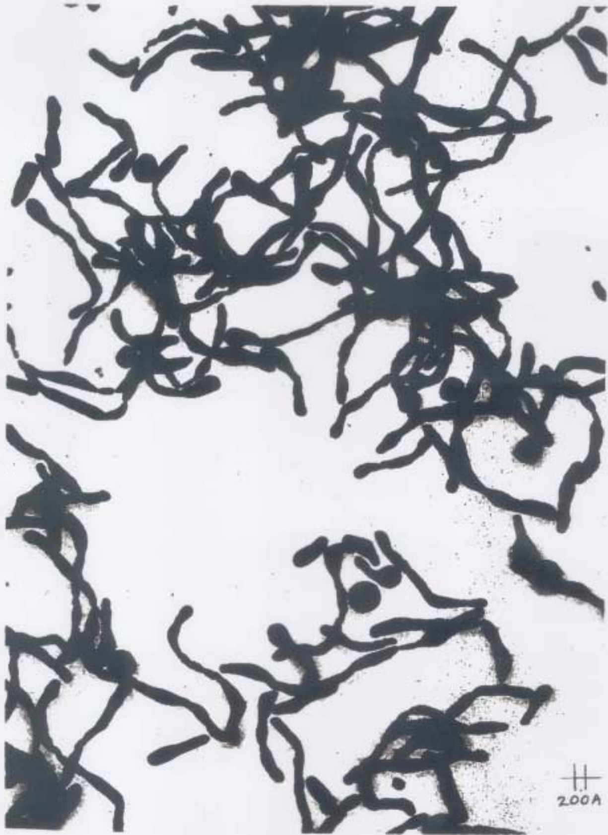
Filamentary silver produced by developing a photographic emulsion.
